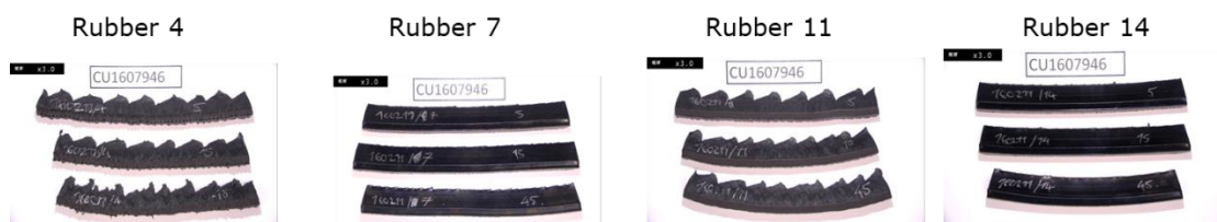
FIGURE 5: Gavey die evaluation from 4 rubber compounds at one throughput – shear rate
