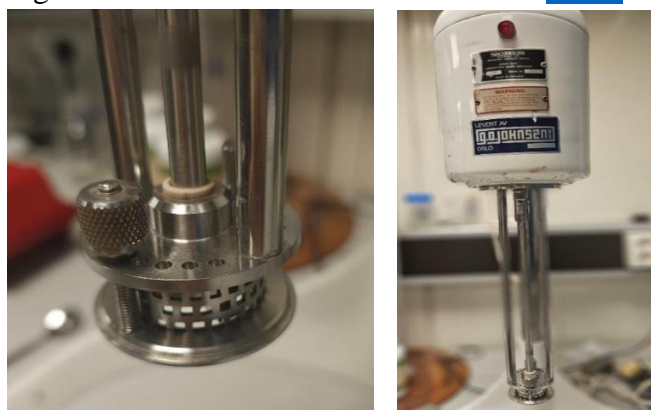
FIGURE 1: Blade used to shear the fluid during drilling fluid preparation
