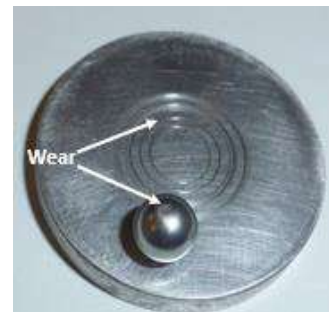
FIGURE 13: Photograph picture of ball-surface wear
