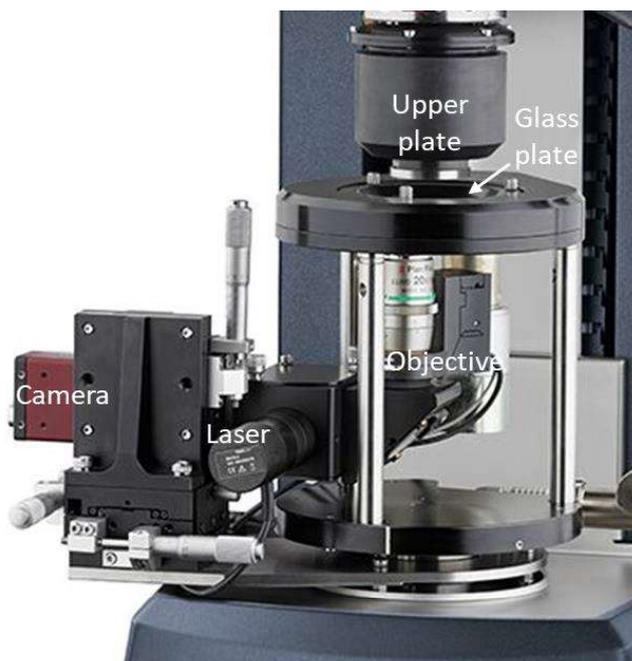
**FIGURE 1:** Experimental setup of the Modular Microscope Accessory mounted in the rheometer.
